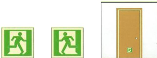
For compliant placement of running man symbol, consult your applicable local or national codes (2009, 2012 IBC section 1024 + 2015 IBC section 1025).
