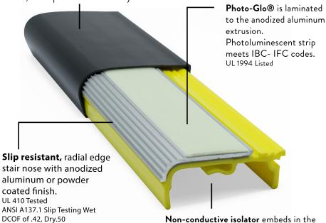
Non-conductive isolator embeds in the wet concrete and remains firmly anchored.
