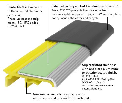
Four piece design; 2" non-conductive pvc isolator, replaceable anodized nosing, replaceable 1" Photo-Glo® strip, patented construction cover. Up to 12 feet, to the nearest 1/16 inch.
